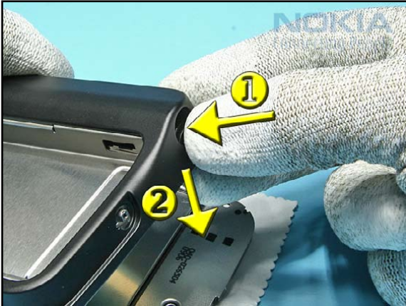
13. First push in the CAMERA MODULE and then pull it out from its place.
