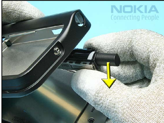
14. Carefully, place the ENGINE MODULE with the CAMERA MODULE onto DISPLAY SHIELD ASSEMBLY.
