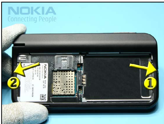
4. Undo the two Torx Plus size 4 screws in the order shown.
