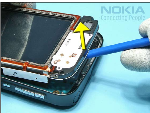
11. Lift the DISPLAY SHIELD ASSEMBLY a bit with the SS-93.
