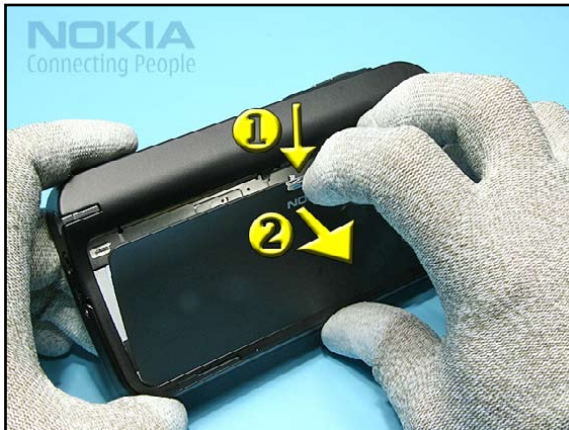
2. Press the RELEASE BUTTON and remove the BATTERY COVER ASSEMBLY. Remove the BATTERY if inserted.
