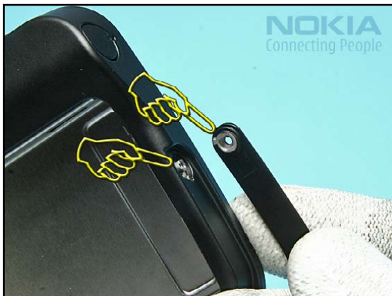
6. Remove the STANDING SUPPORT PAINTED. Note the correct position when assembling the unit.
