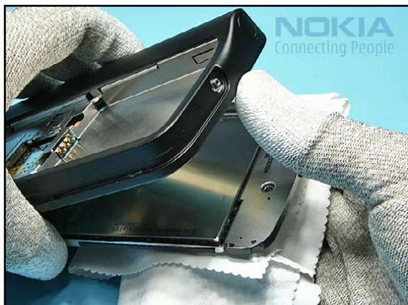
12. Carefully, turn the unit as shown by securing the LCD with a clean cloth.
