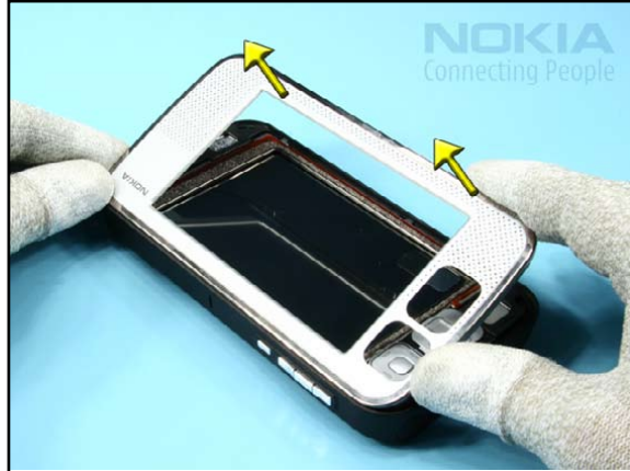
8. Lift the shown side of the A-COVER and remove it carefully.
